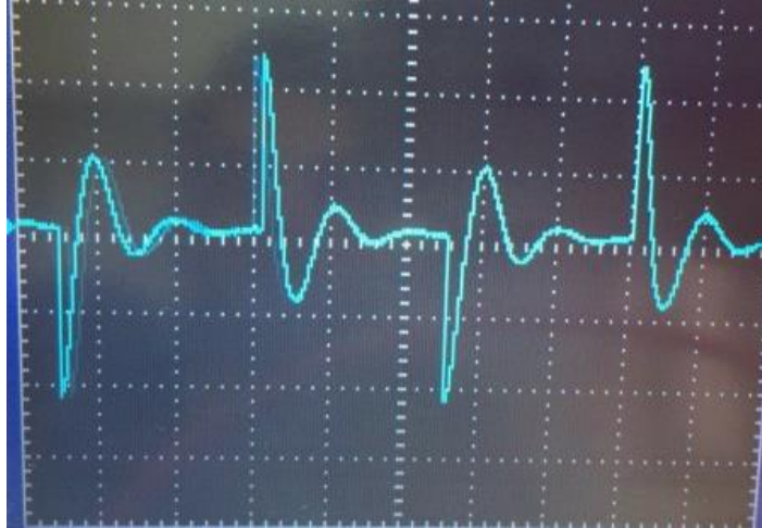
Fig. 2.20: Effect of Changing Derivative Action.
