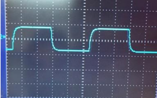
Fig. 2.16: Response of PD Controller for 2 Lag units at gain =50% and T_i of 1
