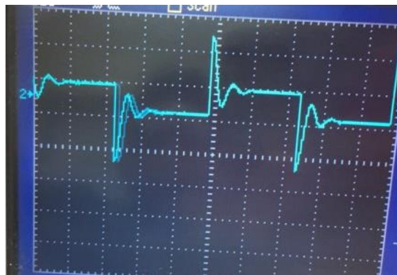
Fig. 2.5: Deviation Signal of P-Controller with Gain =50%
