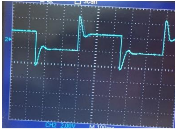
Fig. 2.7: Deviation Signal of P-Controller with Gain =30%
