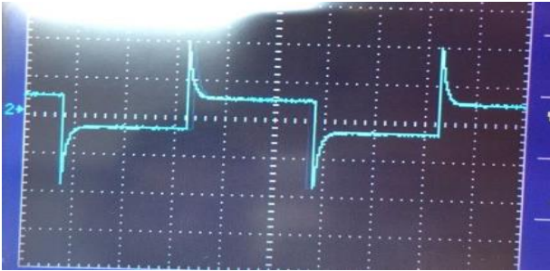
Fig. 2.14: Response of PD Controller for 3 Lag units at gain =50% and T_i of 1
