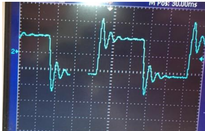
Fig. 2.10: Response of PI Controller for 2 Lag units at gain =50% and T_i of 7
