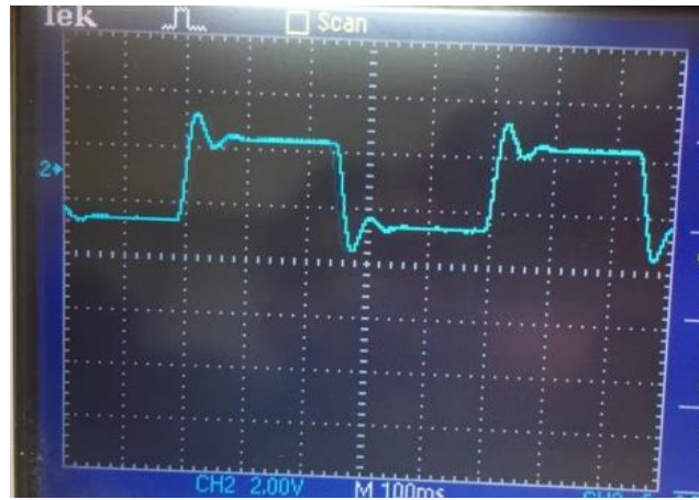
Fig. 2.4: Measured Response of P-Controller with Gain =50%
